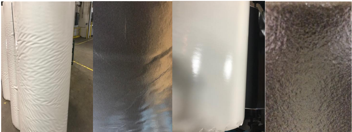
Fig. 1 – Humidity cockles Fig. 2 – Effect on foam Fig. 3 – Smooth inner wind Fig. 4 – Free rise surface
