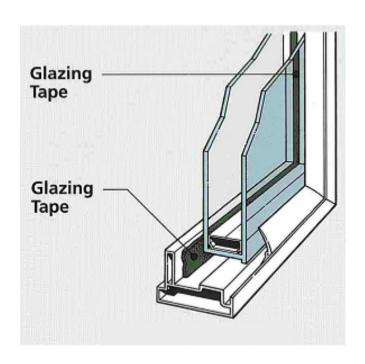
Double faced vinyl glazing tape with aggressive pressure sensitive adhesive on both sides of medium density foam.
