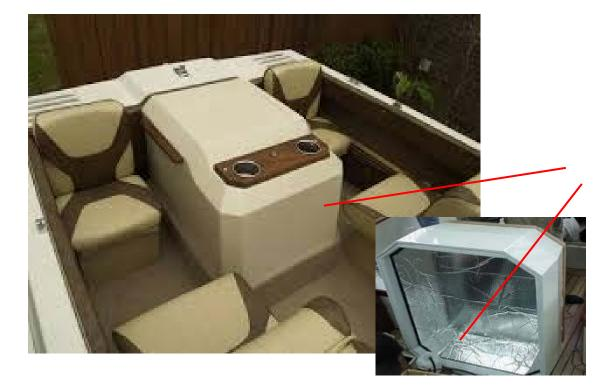
Used on covers and seating area that enclose the inboard motor to reflect heat and insulate.
