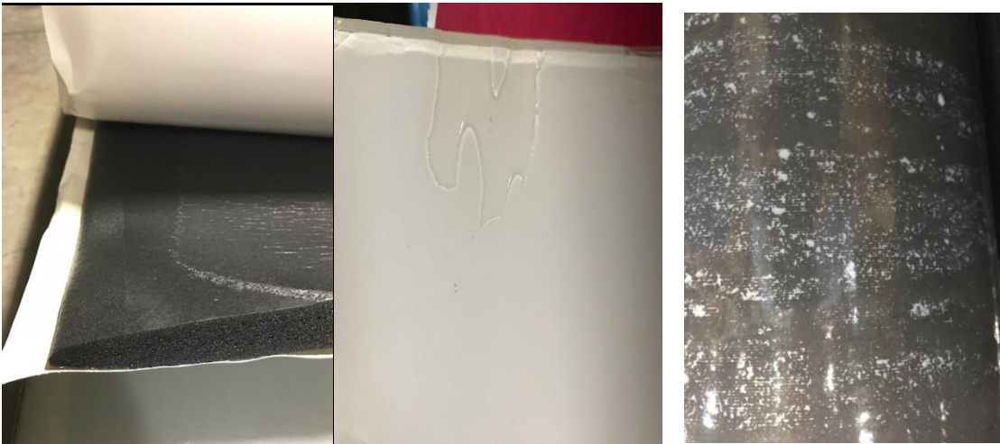
Fig. 8 – Foam drop off effects
