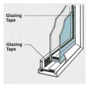
Double faced vinyl glazing tape with aggressive pressure sensitive adhesive on both sides of medium density foam.
