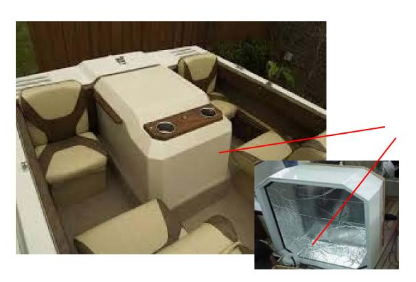
Used on covers and seating area that enclose the inboard motor to reflect heat and insulate.
