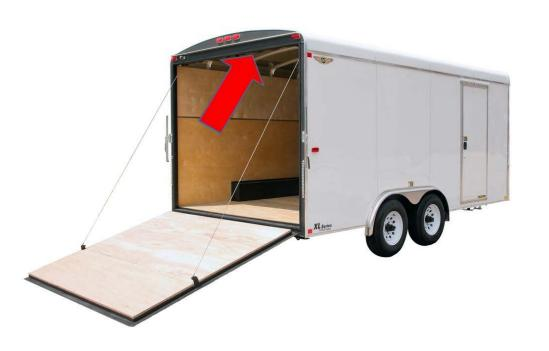
Used for fastening fiberglass roof panels.
